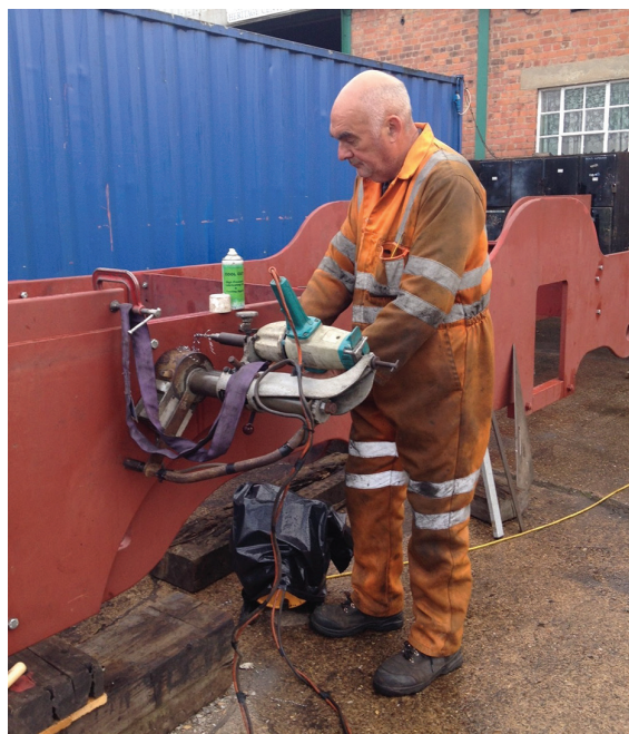
Mike Fairburn drills holes in a doubler plate for assembly onto the frames of No.567. These plates will strengthen the front of the frames, an area of weakness in the original locomotives. SIMON BURTON
