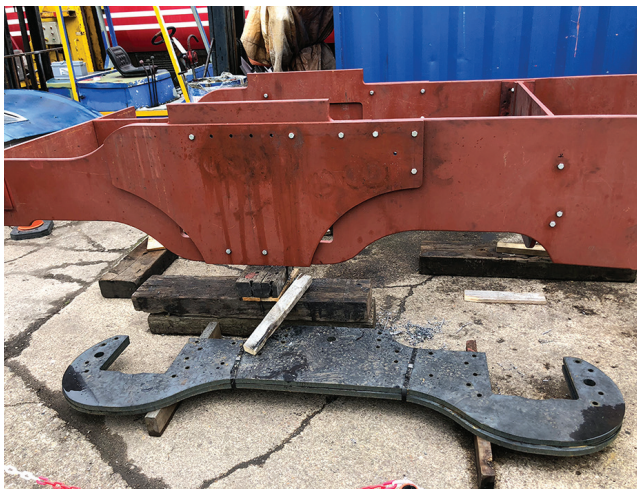
The newly arrived bogie side frames on display at Ruddington, 15th September 2018. ANDREW HORROCKS-TAYLOR
